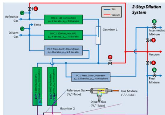
Fig.3: Flow schematics of two-step-diluter, detail: gas mixing device ensuring homogeneous mixtures
