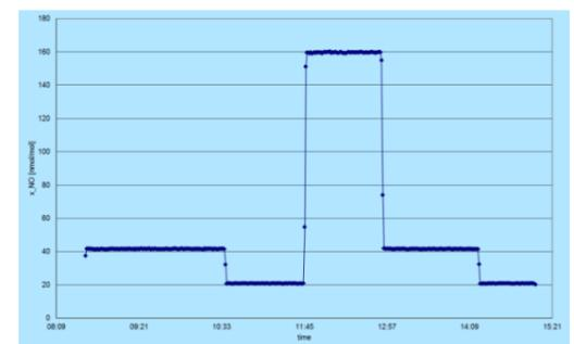
Fig.4: Indicated  $x_{NO}$  values of the repeatability and stability tests at 20, 40 and 160 nmol/mol in nitrogen
