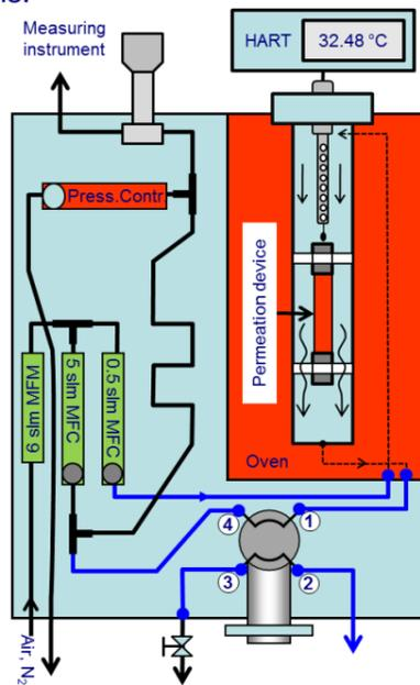
Fig.1: Flow schematics of 'Traceable mobile permeation generator' (TMPG)
