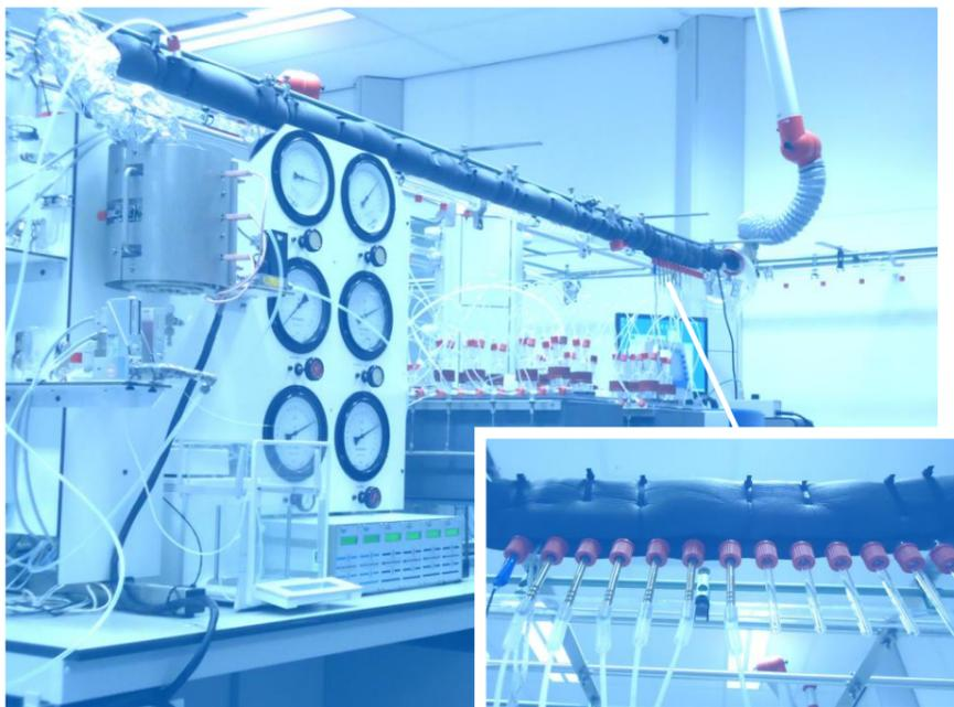
(S)VOC generation system with sampling ports.
