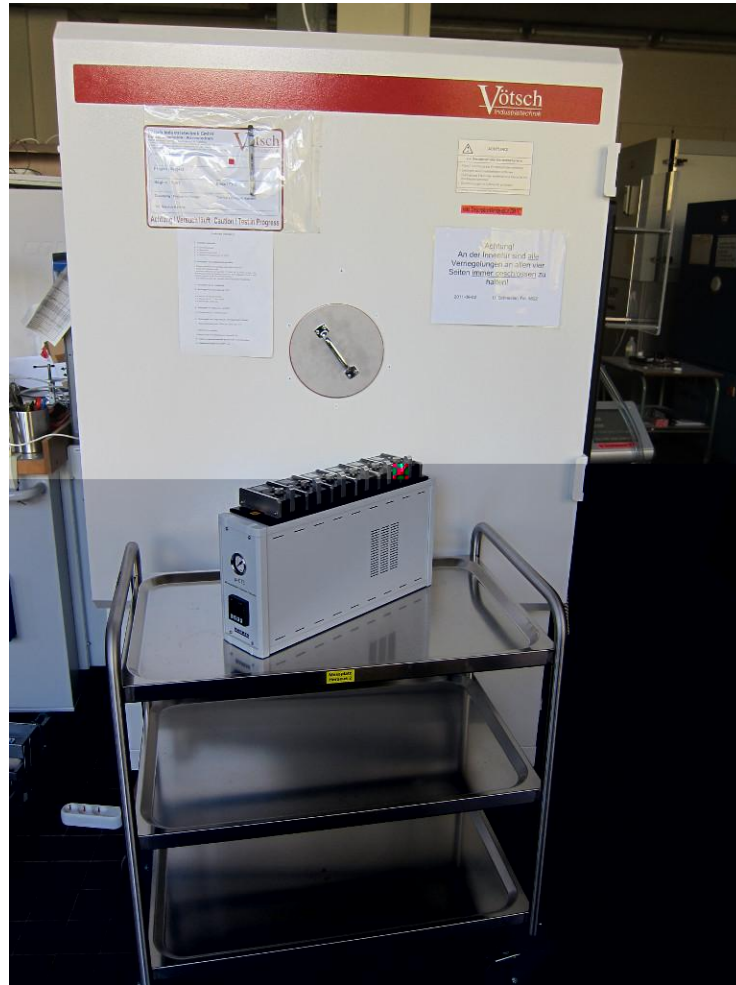
Fig.: size comparison \mu -CTE (front) vs 1-m 3 -chamber (back)
