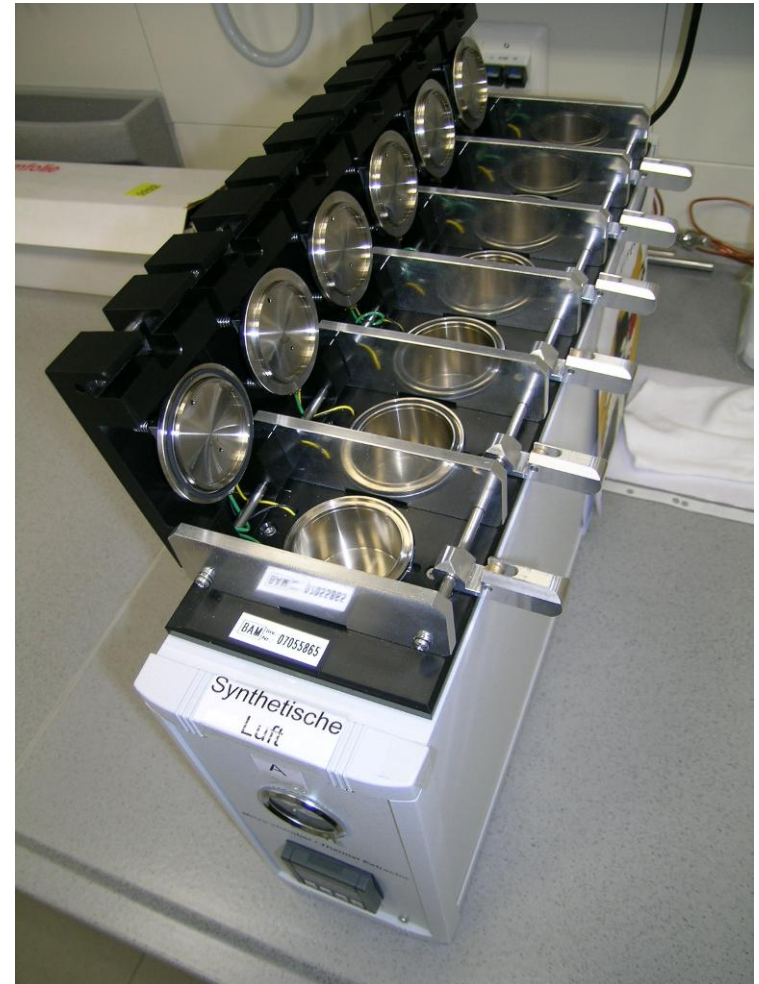
Fig.: Micro-Chamber/Thermal Extractor™ ( \mu -CTE, 44 ml)
