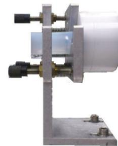
Figure 3 New cell design in which the gas is no longer in contact with metal surfaces.
